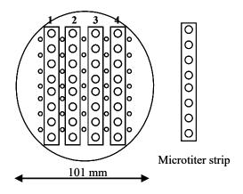
**Figure 9** Schematic drawing of MTIST base plate and microtiter strips.
