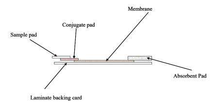
**Figure 26**. Schematic overview of a competitive lateral flow device.
